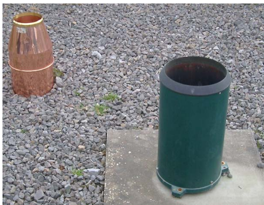
Figure 2 A nonrecording gauge (left) and a recording gauge (tipping bucket) used in the UK
